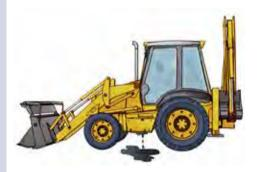
Check tyre condition, tyre pressure and wheel nuts.
