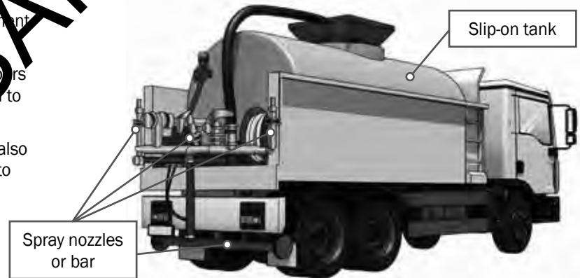
Example of a water vehicle with a slip-on tank
