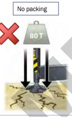
If you **do not** use packing the outriggers could sink and the crane could tip over.
