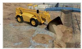
Telehandlers have a telescopic boom, which you can lift, extend and tilt. They have a carriage at the end of the boom. You can quickly fit different attachments to the carriage.
