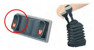
Set the stabilisers down (if fitted). You **must** test raise and lower the work platform before anyone gets into it. This makes sure everything is working properly.
