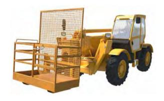
Level the work platform and set the tilt lockout. It automatically keeps the attached work platform level.
