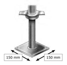
The spindle of an adjustable base plate should extend 150 mm above the maximum nut extension.
