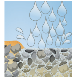
Open Graded Asphalt
