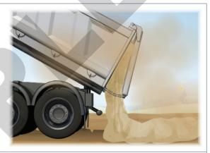
Using a longer chain means more material will flow out.
