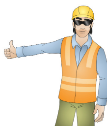
Luffing boom up
