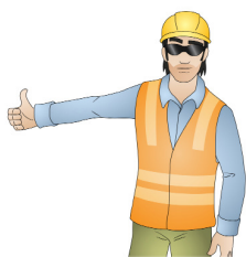
Luffing boom up
