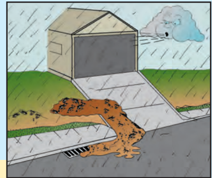
RUN OFF FROM LAND EROSION
