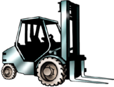
A four wheel drive (4WD) forklift
