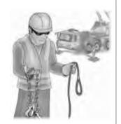
Does the crane and equipment have enough capacity to carry the load? Check the SWL.
