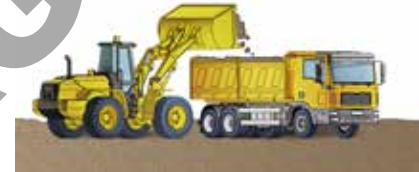
loader and dump truck
