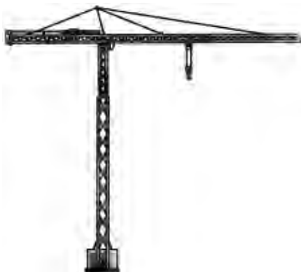
Hammerhead tower crane
