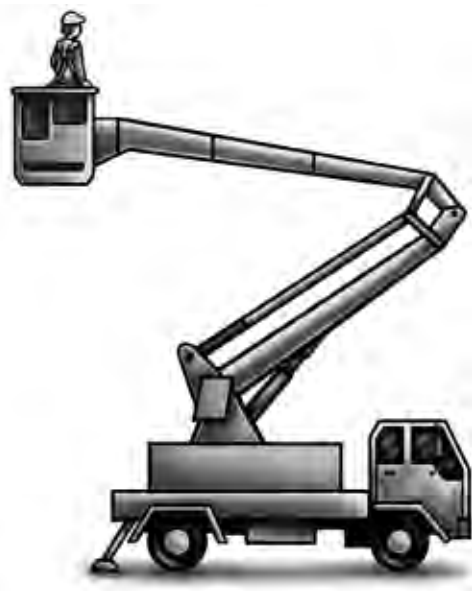
Elevating work platform
