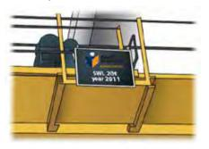
Do not attempt to lift a load which is heavier than the cranes SWL or maximum capacity.
