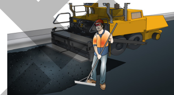
1. Stand at edge of asphalt area
