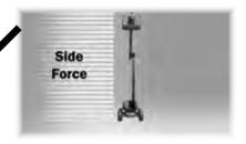
Wind load is the maximum wind speed at which the EWP can work safely. The maximum wind load for he EWP you are using should be in the EWPs persual to on the EWP itself.
