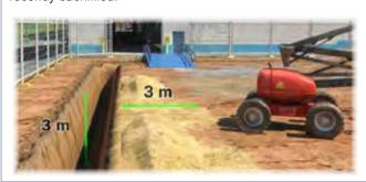
If you set up too close to a trench, or the ground is too soft the side of the trench might collapse and cause the EWP to tip over.
