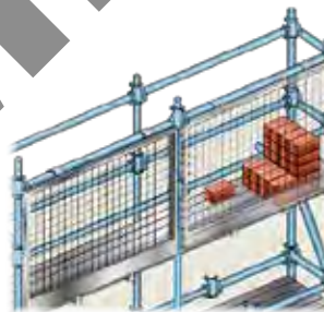
Store materials on overhead gantries.
