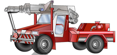
Non-slewing mobile crane
