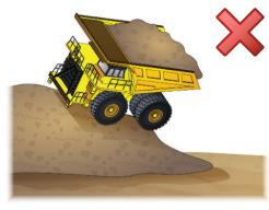
Don't dump while the truck is on a slope.
