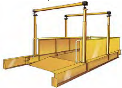
Rigging of cantilevered platforms (personnel and materials hoist)
