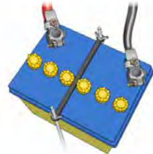
Check that the battery is secure, connected properly and the fluid level is correct.
