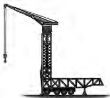
Self erecting tower crane
