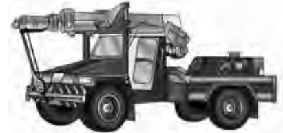
Non-slewing mobile crane
