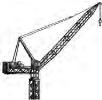
Luffing boom crane
