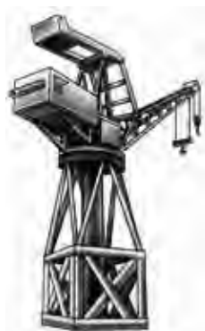
Portal boom crane
